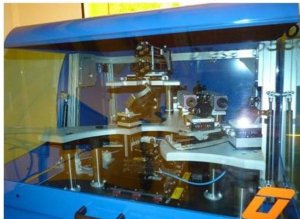
**Figure 9:** A photography of the DILASE 650 KLOE instrument used to fabricate micro-gears, micro-beams and anchoring pads.
