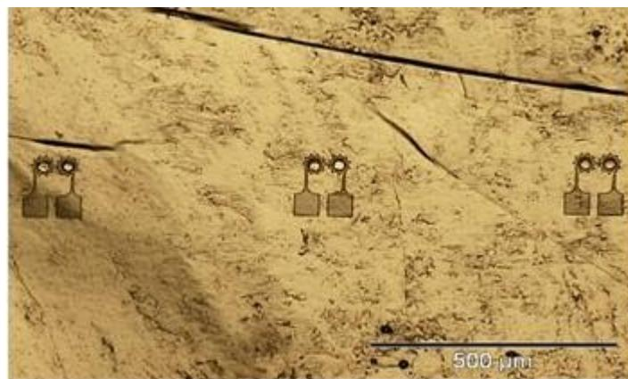
*Figure 19: Optical microscope image of a series of three 2 stages mechanical calculator with Ni micro-axle micro-lithographed on the graphite/SiO<sub>2</sub>/Si surface. The cleanness of the graphite surface has still to be improved.*
